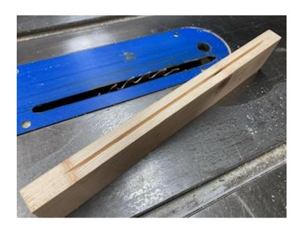
Construct the doors using standard 1" x 4" boards. Rip them down to 2" wide strips. Cut to length as follows: four pieces at 20" long, and four pieces at 11 %" long. Cut a dado into the inside edge of the frame to accommodate the plexiglass window, about ¼" deep.
